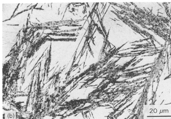
Figure 2 OM micrographs of bainitic structure of 60 C and 60 CSM steels, transformed isothermally (IT) at 673 K. Specimens were etched by 5 vol% nitrate alcohol solution. (a) 60 C steel (IT for 50 s); (b) 60 CSM steel (IT for 30 s).
